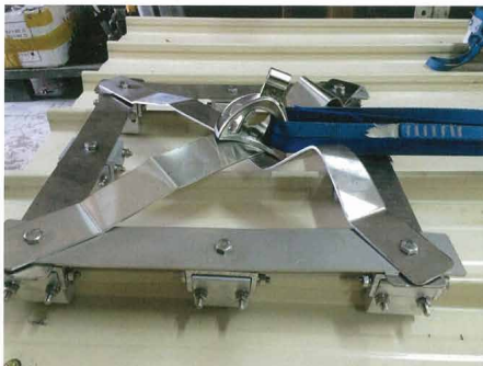
Photograph 5: Shows the Fall Arrest System (End Spider) with AK Clamps (X8) MTL ALUM pulled Parallel to the roof seam at force of 1219kg
