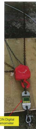
Photograph 4: Shows direction of pulling & the Force of the Fall Arrest System with AK Clamps MTL ALUM Parallel to the roof seam
