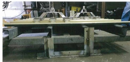
Photograph 2: Shows test bed of the Fall Arrest System (End Spider) with AK Clamps (X8) MTL ALUM installed Perpendicular & Parallel to the roof seam - (Front View)
