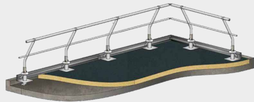
Guard Rail for Roof Slab (to be sealed)
